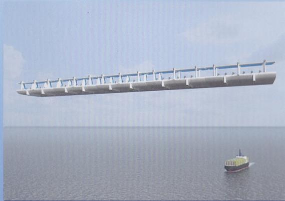
ConcordLift™ is a configuration. It is a tandem wing aircraft (without fuselage) that provides stability and extra lift for a cargo airfoil pod.
